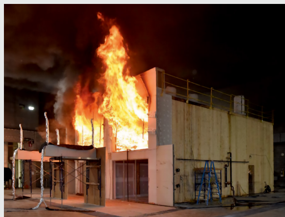
Compartment fire testing of a two-story mass timber building as part of the 2017 ATF fire tests in Washington D.C. Image Source: American Wood Council
