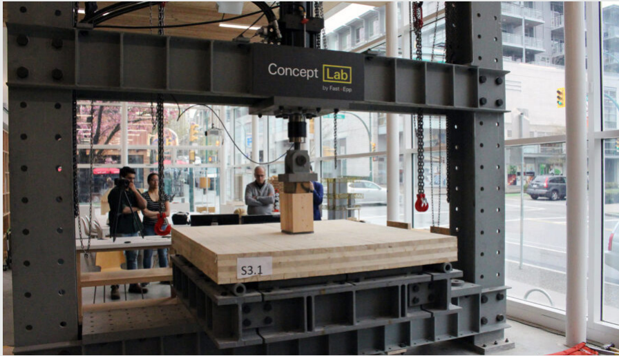
Image of tests conducted by Fast + Epp on CLT minor strength axis moment connections in their Concept Lab. Source image: Fast + Epp, 2024.
