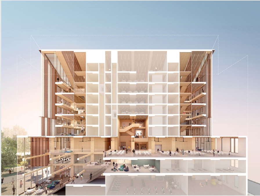
Limberlost Place, a ten-storey exposed mass timber building designed by Moriama Teshima Architects with Acton Ostry Architects for George Brown College in Toronto. This pioneering structure features assembly spaces throughout its full height while achieving net-zero carbon emissions. Source image: Moriama Teshima Architects.
